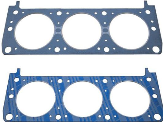
In some cases, head gaskets or intake manifold gaskets won't have any directional indicators on them. They may have Blue Stripe® coating or be a different color. In these cases, it does not matter which direction the gasket is installed. If it were crucial, it would be marked.
