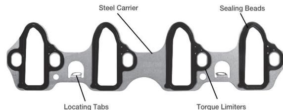
The metal carrier design of MS 98016 T also incorporates locating tabs that hold the gasket in place on the cylinder head by slipping over the head bolts. This is a more durable solution than the OE plastic clips.
