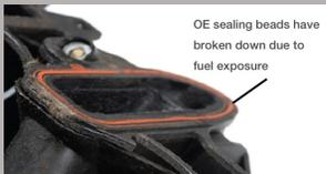
OE sealing beads have broken down due to fuel exposure
