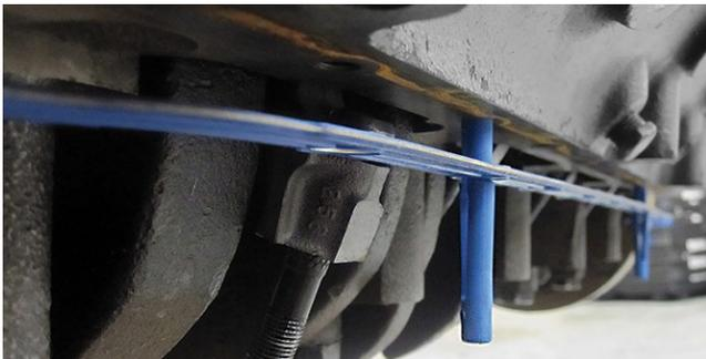
Fel-Pro has developed an innovative and easy solution to these issues. Fel-Pro oil pan SnapUps are the clean, simple and effective way to speed up an oil pan gasket replacement. Simply thread them into the block where the oil pan bolts go, snap the oil pan gasket in place, followed by the pan itself, and start threading the bolts in. Once the oil pan is secure, the SnapUps are easily removed and are reusable.
