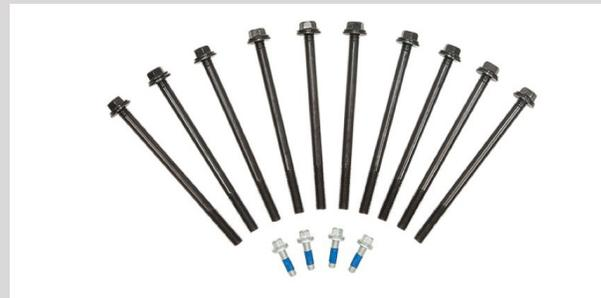
When T-T-Y bolts are rotated to their final number of degrees of rotation, T-T-Y bolts can approach their elastic limit and become permanently stretched. If removed and reused, it is likely that either the head gasket will fail (due to low clamp load) or the bolts will break.
