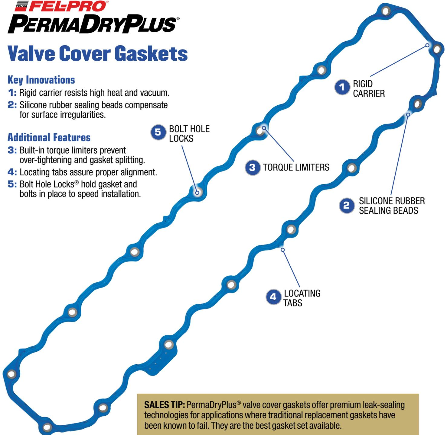
**SALES TIP:** PermaDryPlus® valve cover gaskets offer premium leak-sealing technologies for applications where traditional replacement gaskets have been known to fail. They are the best gasket set available.
