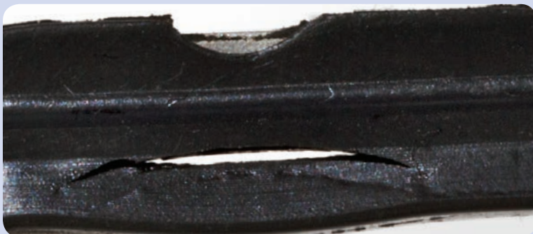
“Other” gasket part began leaking coolant at 140 hours.
