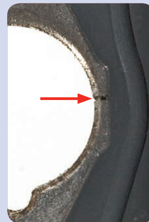
“Other” Gasket (crack at compression limiter)
