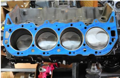
THE COOLANT HOLES IN THE BLOCK CASTING ARE MUCH LARGER THAN THOSE IN THE FEL-PRO HEAD GASKET – THIS IS BY DESIGN!
