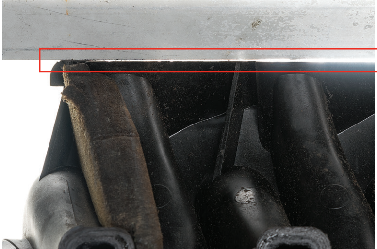
Light visible between straight-edge and port sealing surfaces indicates manifold warpage
