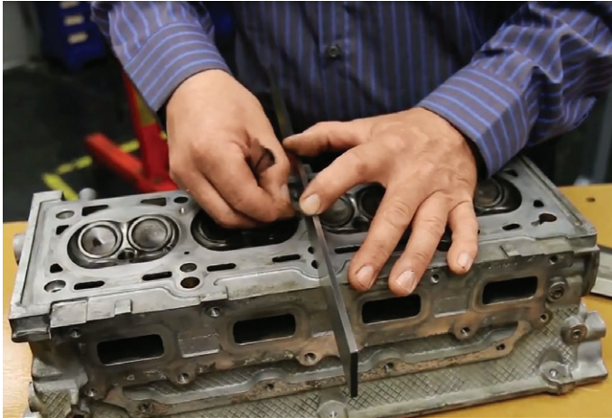
John Gurnig checking flatness across an inline-4 cylinder head in the Fel-Pro Field Test Garage
