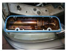
PermaDry® gasket installed dry
