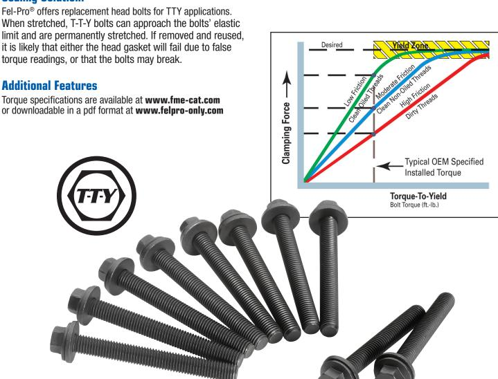
**SALES TIP:** ALWAYS recommend new Fel-Pro Torque-to-Yield head bolts when you sell a new Fel-Pro head gasket! There is no way to tell if head bolts have been previously removed or installed, so suggest replacement.
