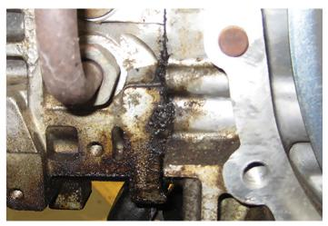
Fig 1. External oil leak from failed gasket
