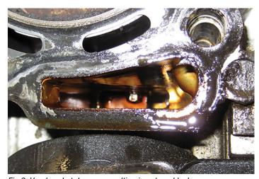
Fig 2. Head gasket damage resulting in external leak
