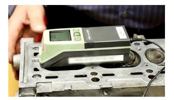
In order to determine an appropriate surface finish, consider the metallurgy of the head and block castings as well as the material and design of the head gasket being used in the install. **Different gaskets require different surface finishes,** so the surface finish must be matched to the type of gasket that is required for the application. To determine surface finish requirements, consult the OEM repair manual.
