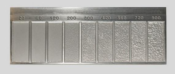
**Roughness Average (Ra)** is the average micro-inch measurement of peak-to-valley roughness height of a flat surface. The lower the Ra number, the smoother the surface. Fel-Pro recommends a finish of 60 to 80 Ra for cast iron cylinder heads and blocks and 50 to 60 Ra for aluminum.
