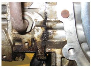
External oil leak from failed head gasket
