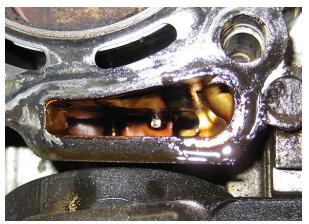
Head gasket damage, resulting in external leak
